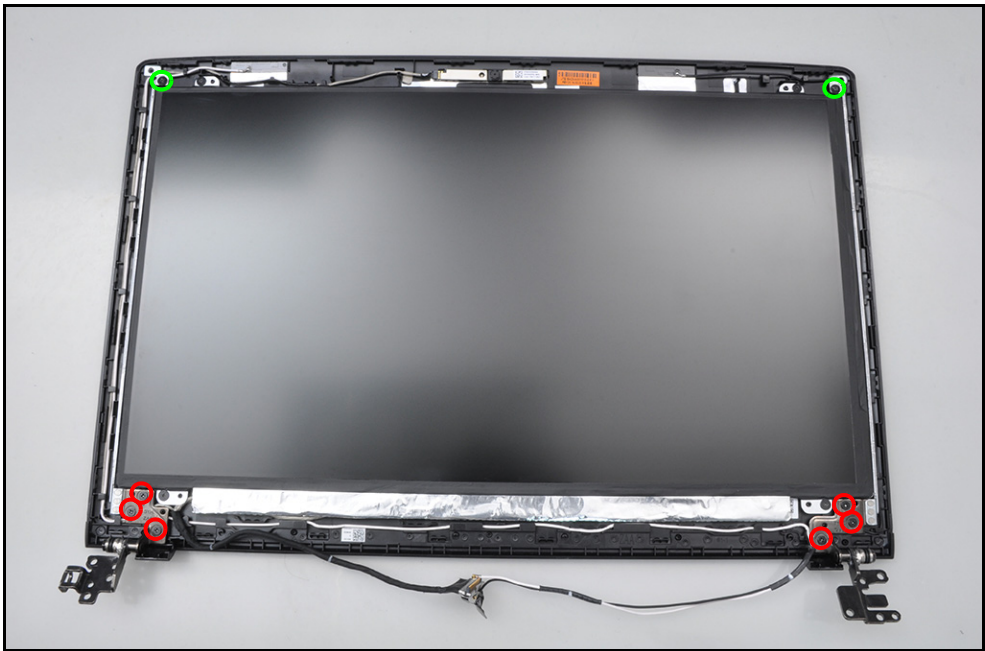
Figure 3-79. Replacing the LCD Hinges
