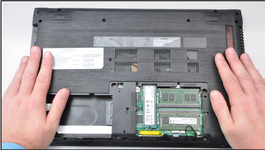
Figure 3-110. Replacing the Base Cover
