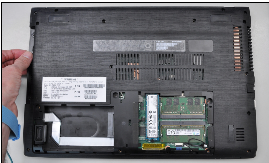
Figure 3-19. Base Cover Removal
