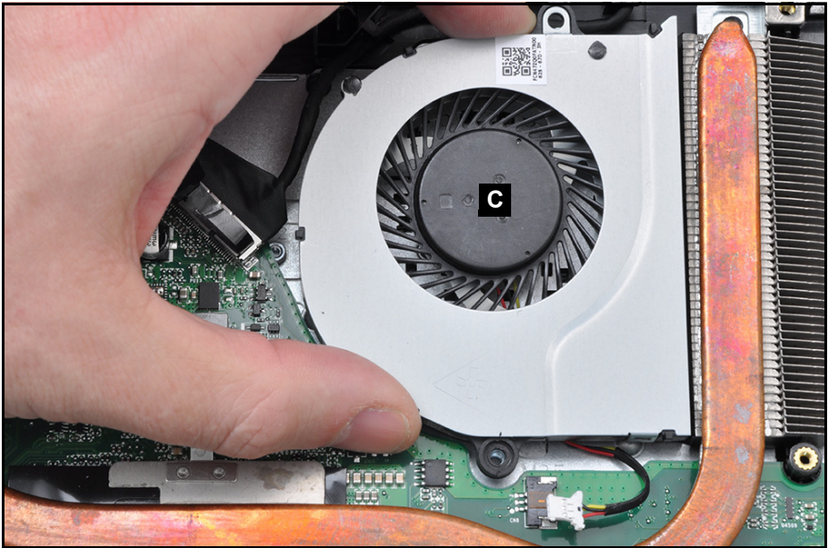
Figure 3-32. Fan Removal
