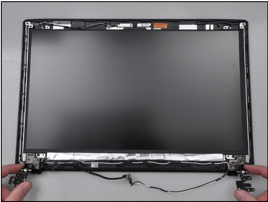
Figure 3-64. LCD Hinge Removal
