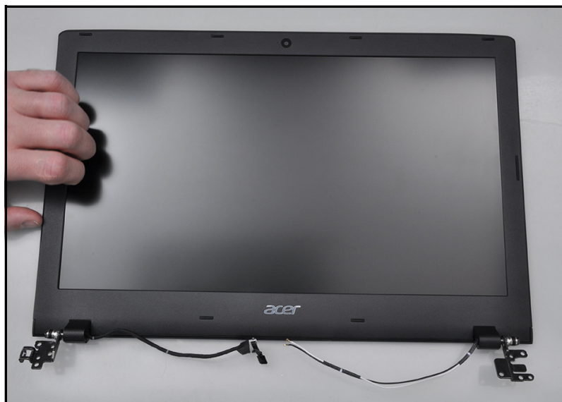
Figure 3-55. LCD Bezel Removal
