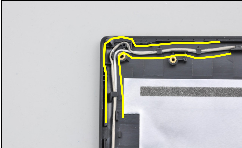
Figure 3-75. Replacing the eDP & Camera Cable
