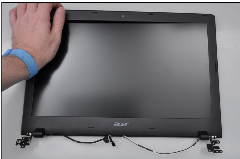
Figure 3-54. LCD Bezel Removal
