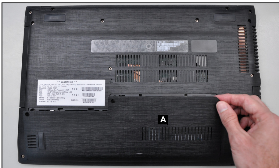
Figure 3-118. Replacing the HDD Door
