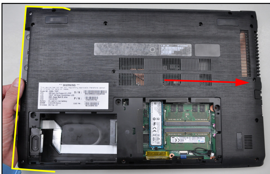
Figure 3-20. Base Cover Removal
