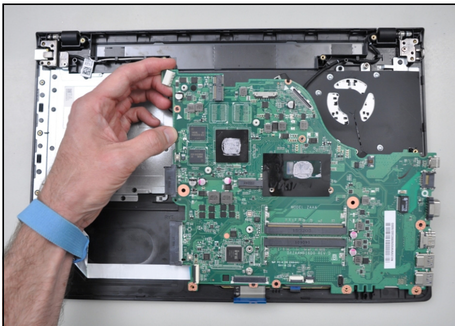
Figure 3-39. Mainboard Removal
