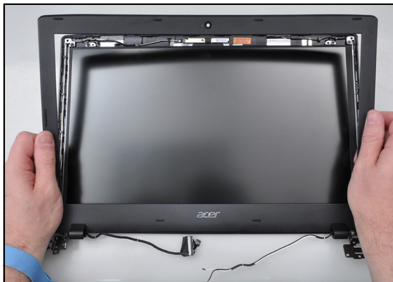
Figure 3-57. LCD Bezel Removal
