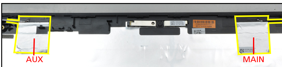
Figure 3-68. WLAN Antenna Removal
