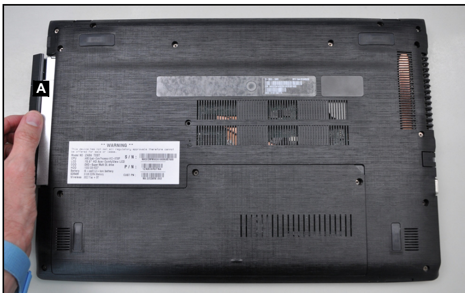
Figure 3-4. ODD Module Removal
