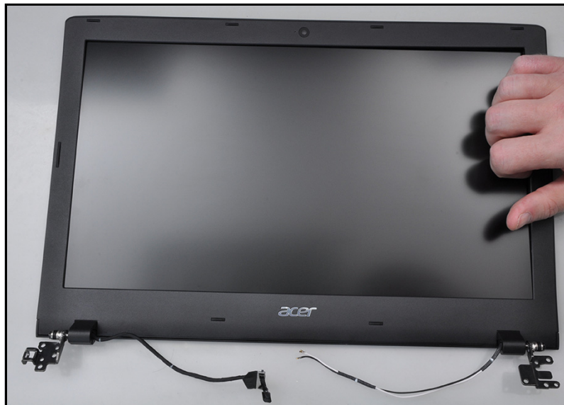
Figure 3-56. LCD Bezel Removal
