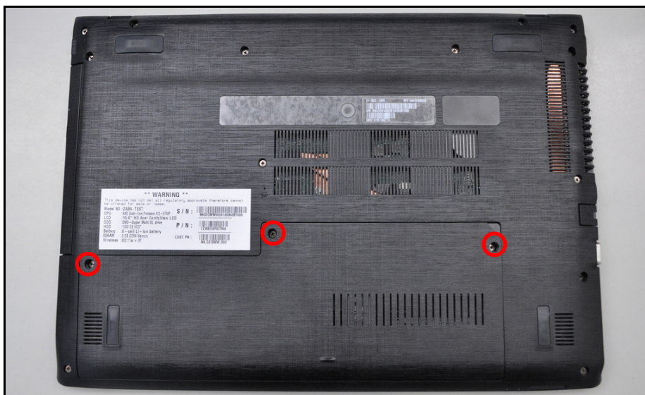
Figure 3-119. Replacing the HDD Door
