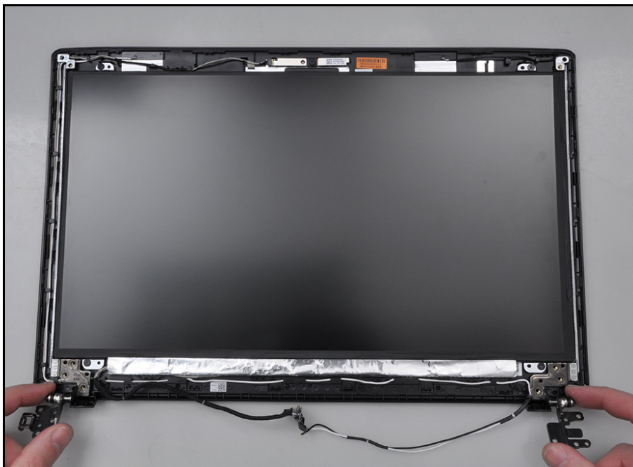
Figure 3-78. Replacing the LCD Hinges
