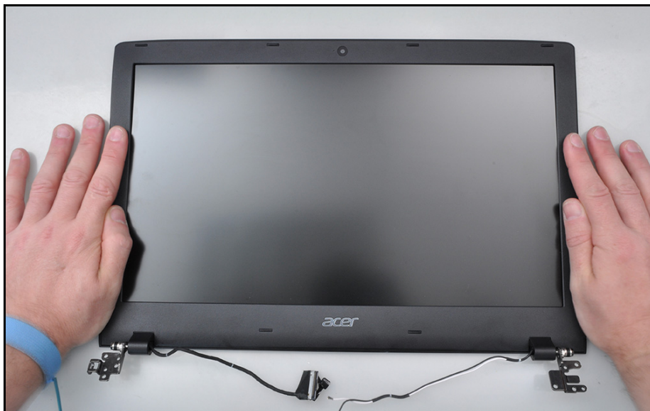
Figure 3-84. Replacing the LCD Bezel
