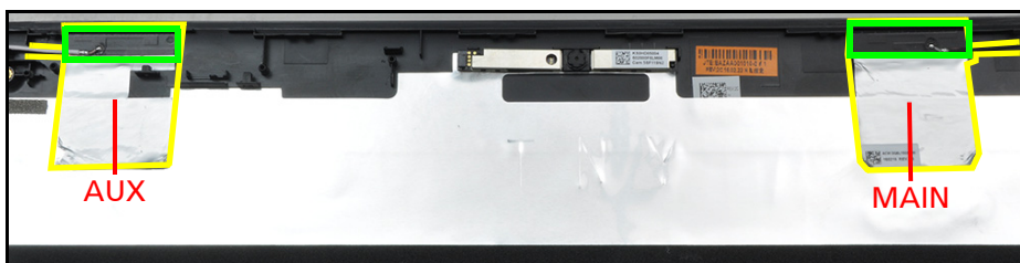
Figure 3-70. Replacing the WLAN Antenna
