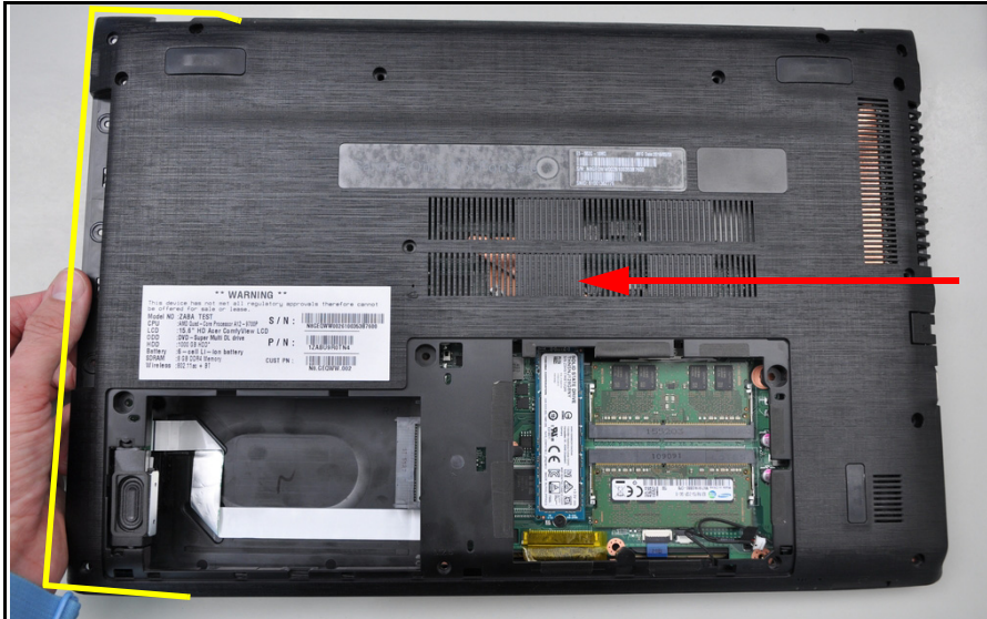
Figure 3-109. Replacing the Base Cover
