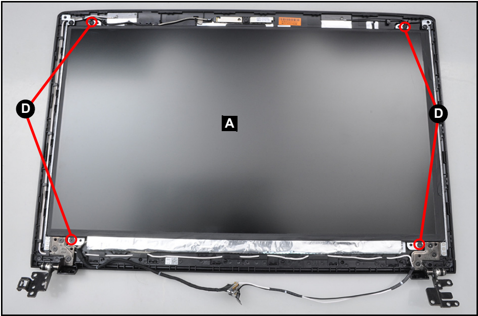
Figure 3-82. Replacing the LCD Panel
